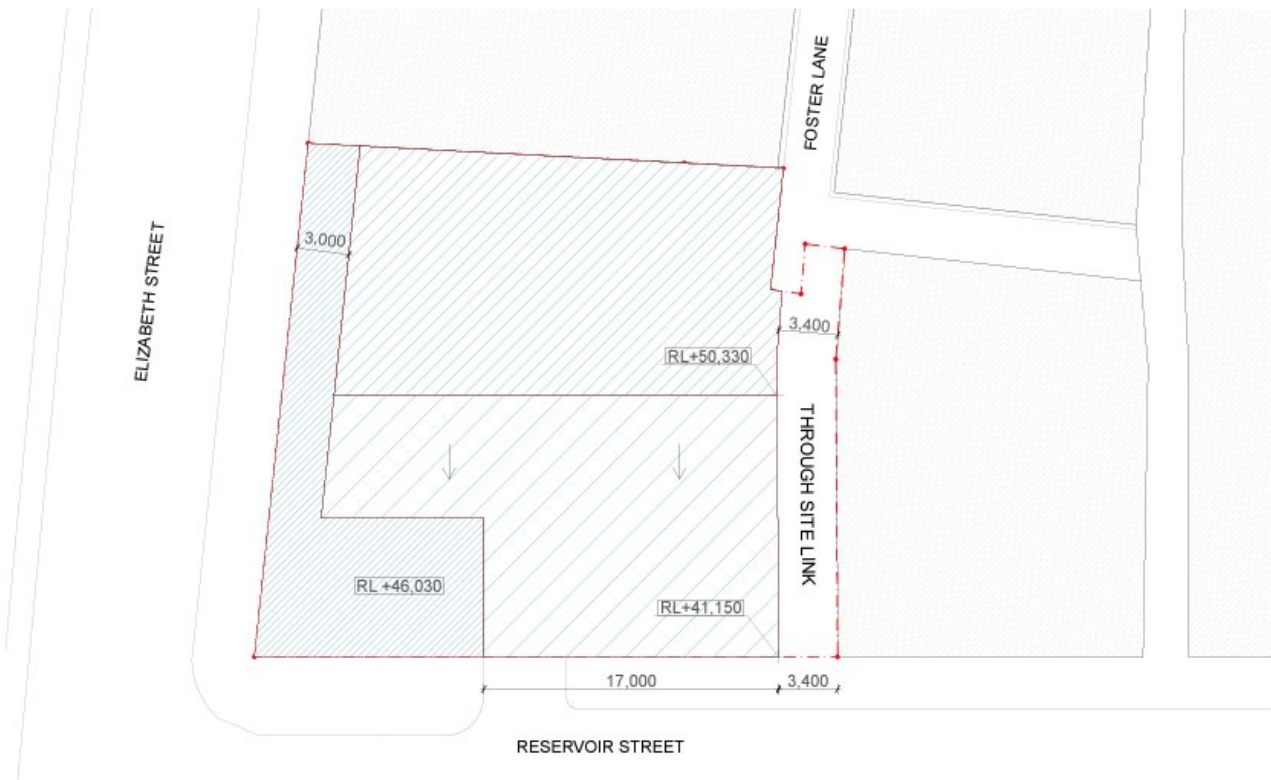
Figure 16. Proposed building envelope – roof plan
